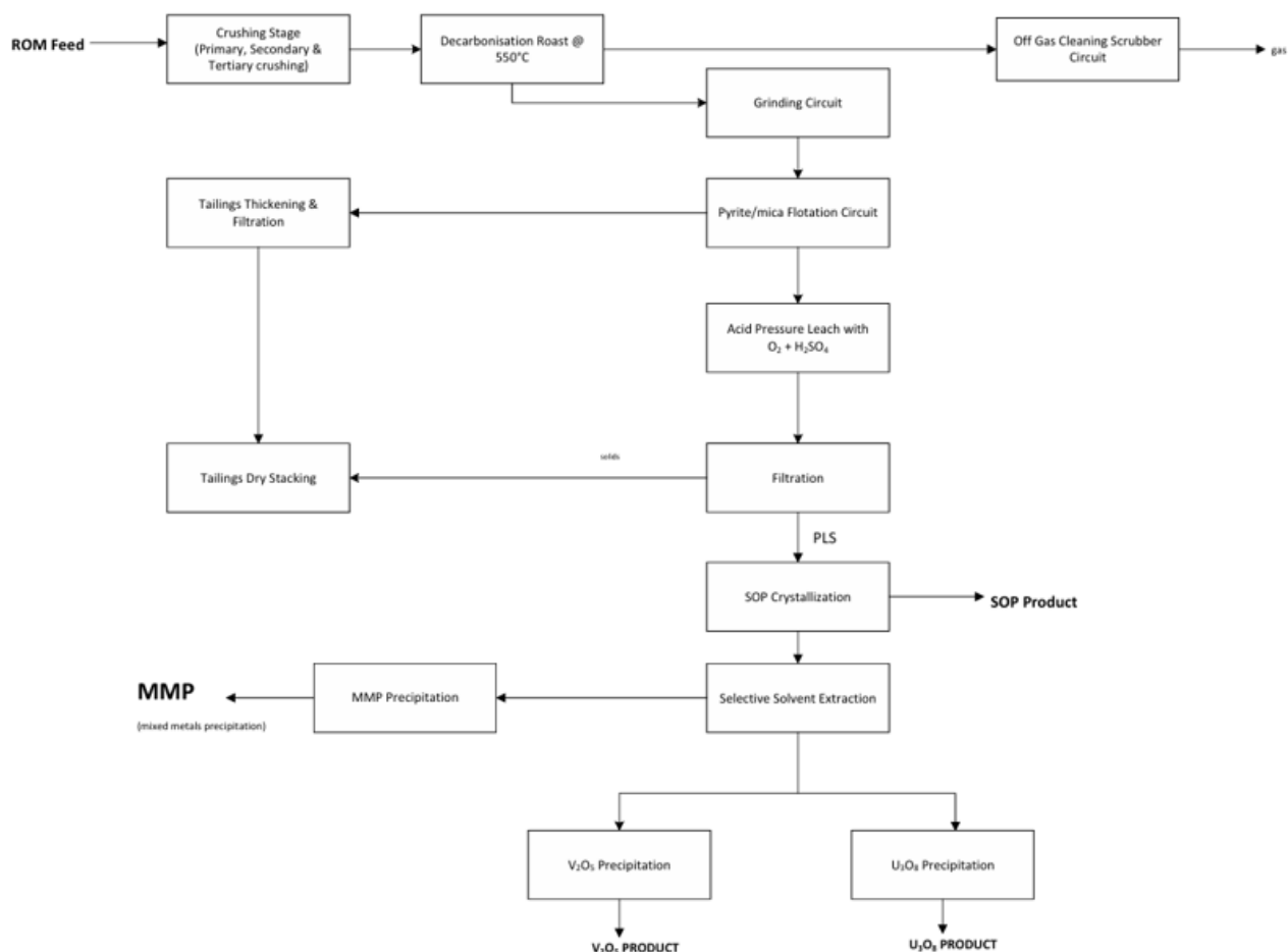
FIGURE 24.2 BLOCK FLOW DIAGRAM ACID PRESSURE LEACH
