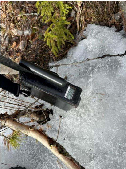
FIGURE 12.13 SCINTILLOMETER SHOWING READING TAKEN AT SHALE OUTCROP 1
