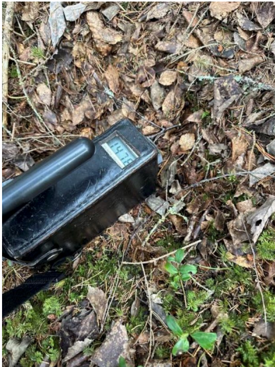
FIGURE 12.16 STOP 5: SCINTILLOMETER SHOWING READING TAKEN AT SHALE OUTCROP 2
