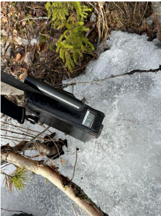
FIGURE 12.13 VIKEN TOUR STOP 4: SCINTILLOMETER SHOWING READING TAKEN AT SHALE OUTCROP 1
